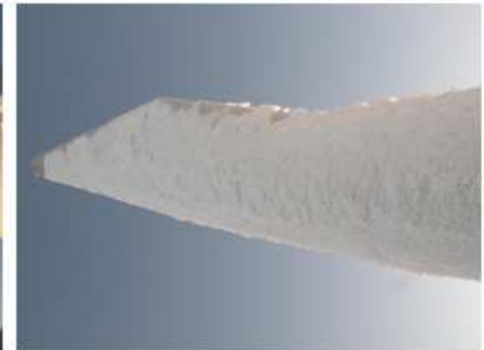
Turbine 2 - Ice prevention system fault
